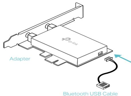
c. Locate an available **PCIe slot ( X1, X4, X8, or X16)** and carefully insert the adapter.
